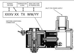
The coil 30XDM Exdm is developed to fit Amisco operators. If a different operator is used, make sure that the coil powered with nominal voltage does not show a power consumption exceeding the values mentioned above
